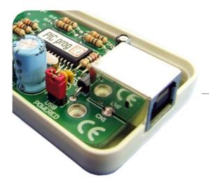
This picture shows the position of jumper when the target board and *PICflash* programmer are powered trough USB connector.
