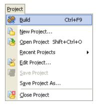
Compiler will generate output files in the project folder. There should be 4 new files: ProjectName.asm, ProjectName.lst, ProjectName.mcl, and ProjectName.hex. The last one will be used to program the microcontroller directly.
