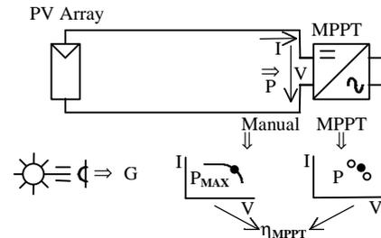
**Figure 8:** Using manual mode to obtain I-V curve data
