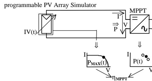
**Figure 4:** Dynamic laboratory measurements
