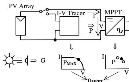
Figure 5: Switching between inverter and IV tracer
